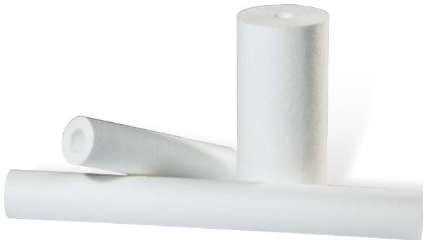
PP material is molten and directly sprayed with high temperature and pressure to be three-layer structure. Filter is inside with dense fibers and outside with loose ones. This design allows it to capture particles of varying sizes. The usability of this melt-blown filter make them the ideal pre-filters for most industrial processes.
